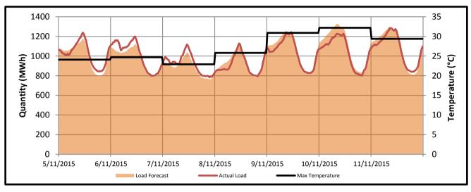
The maximum temperatures for this trading week ranged from  $22.9^{\circ}$ C to  $32.2^{\circ}$ C. The actual load peaked at 1284.388 MWh on the 11/11/2015.
