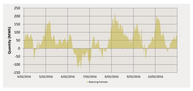
The majority of the balancing activity this week occurred within Balancing Demand. The maximum balancing demand for the week reached 210.738 MWh on the 8/2/2016. The maximum balancing supply for the week reached -123.378 MWh on the 6/2/2012.
