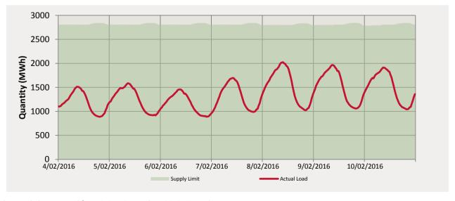
The supply limit ranged from 2787.727 MWh to 2840.42 MWh
