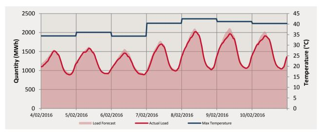
The maximum temperatures for this trading week ranged from  $34.3^{\circ}$ C to  $42.5^{\circ}$ C. The actual load peaked at 2023.347 MWh on the 8/2/2016.
