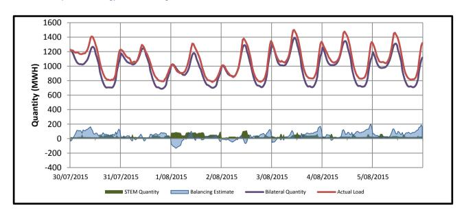
Total balancing supply equalled -2345.291 MWh whereas total balancing demand equalled 16508.387 MWh. The Total STEM Traded quantity was 12445.802 MWh, with the STEM Clearing Quantity ranging between 8.99 MWh and 115.66 MWh.
