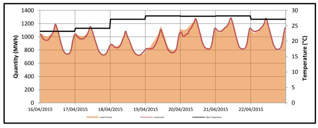
The maximum temperatures for this trading week ranged from  $23.2^{\circ}$ C to  $28.2^{\circ}$ C. The actual load peaked at 1282.301 MWh on the 21/4/2015.
