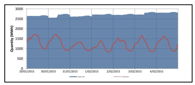
The supply limit ranged from 2557.01 MWh to 2842.274 MWh
