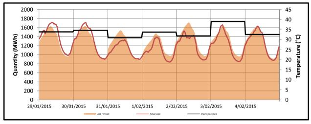
The maximum temperatures for this trading week ranged from  $31^{\circ}$ C to  $39.1^{\circ}$ C. The actual load peaked at 1712.793 MWh on the 30/1/2015.
