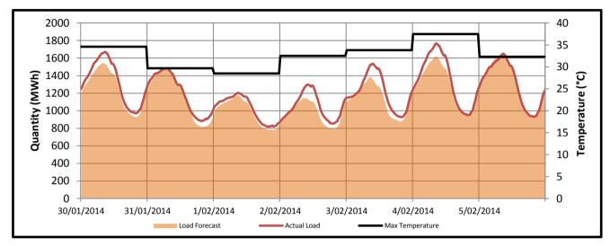
The maximum temperatures for this trading week ranged from 28.5°C to 37.5°C. The actual load peaked at 1767.801 MWh on the 4/2/2014.
