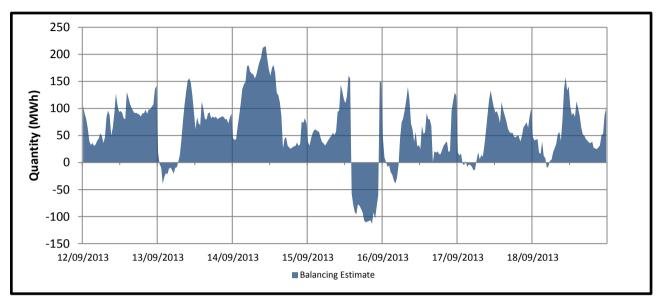
The majority of the balancing activity this week occurred within Balancing Demand. The maximum balancing demand for the week reached 214.768 MWh on the 14/9/2013. The maximum balancing supply for the week reached -113.281 MWh on the 15/9/2012.
