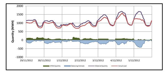
Total balancing supply equalled -45647.84 MWh whereas total balancing demand equalled 20.84 MWh. The Total STEM Traded quantity was 25855.521 MWh, with the STEM Clearing Quantity ranging between 12.232 MWh and 184.668 MWh.
