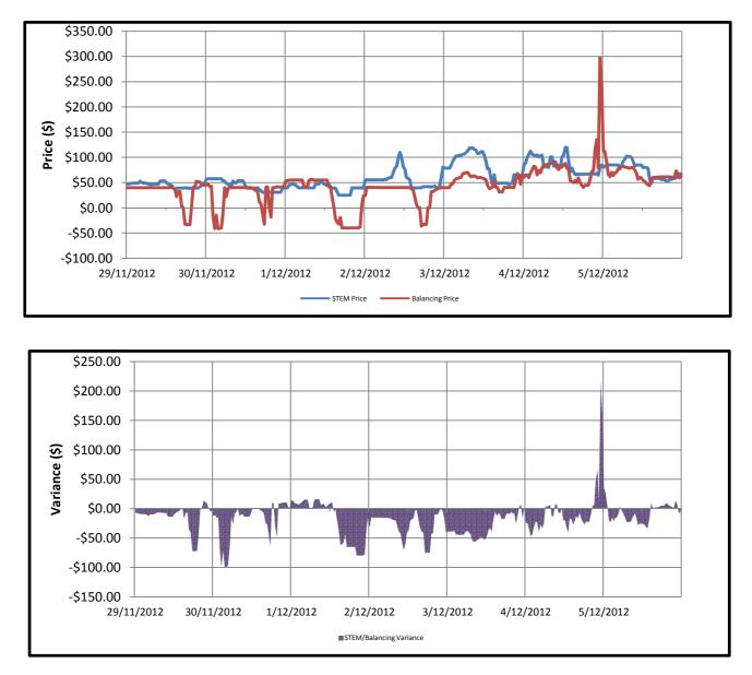
The maximum STEM price was \$119.5/MWh on the 4/12/2012 and the minimum STEM Price recorded was \$25/MWh on the 1/12/2012. The maximum Balancing price was \$297.75/MWh on the 4/12/2012 and the minimum Balancing price recorded was \$-41.33/MWh which occurred on the 30/11/2012.
