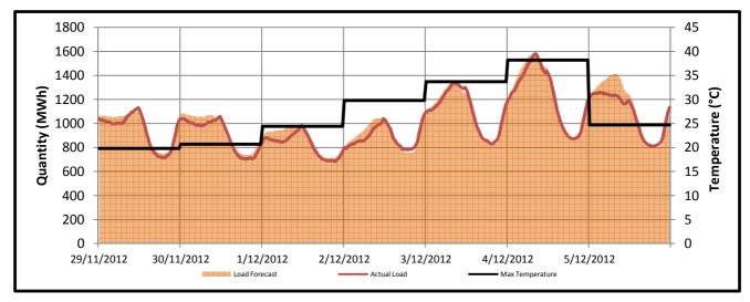
The maximum temperatures for this trading week ranged from 19.8°C to 38.2°C. The actual load peaked at 1579.16 MWh on the 4/12/2012.
