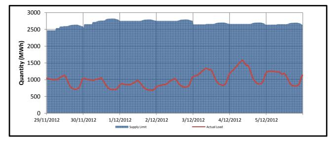
The supply limit ranged from 2472.973 MWh to 2824.404 MWh
