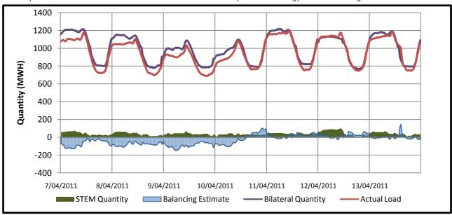
Total balancing supply equalled -13919.38 MWh whereas total balancing demand equalled 3717.96 MWh. The Total STEM Traded quantity was 13896.369 MWh, with the STEM Clearing Quantity ranging between 5.295 MWh and 102.469 MWh.
