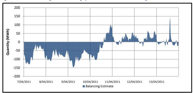
The majority of the balancing activity this week occurred within Balancing Supply. The maximum balancing demand for the week reached 146.749 MWh on the 13/4/2011. The maximum balancing supply for the week reached -148.52 MWh on the 9/4/2011.
