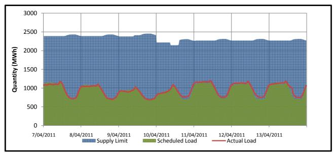
The supply limit ranged from 2144.944 MWh to 2456.334 MWh with the Scheduled System Load peaking at 1155.812 MWh on the 7/4/2011.
