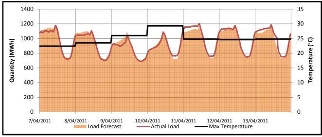
The maximum temperatures for this trading week ranged from  $22.4^{\circ}C$  to  $29.3^{\circ}C$ . The actual load peaked at 1201.215 MWh on the 11/4/2011.
