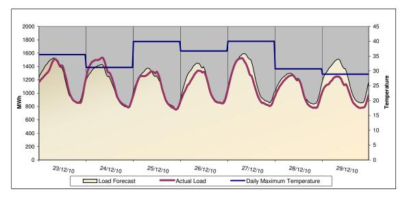
The maximum temperatures for this trading week ranged from  $28.9^{\circ}$ C to  $40.0^{\circ}$ C. The actual load peaked at 1,533 MWh on the 24/12/10. The actual load mirrored the forecast load for most of the week.
