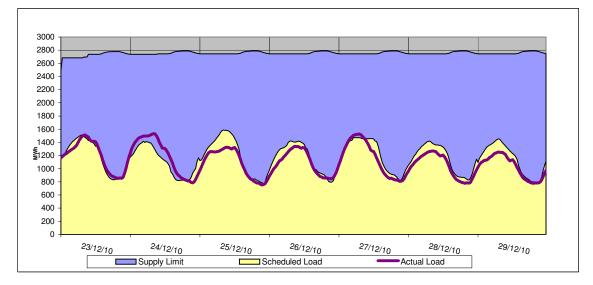
The supply limit was fairly consistent during the course of the week. The supply limit ranged from 2,486 MWh to 2,788 MWh with the actual load deviating from the Scheduled System Load for most of the week.
