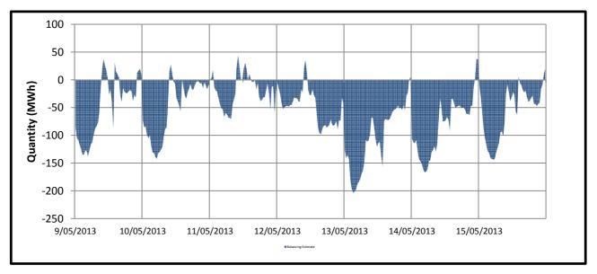
The majority of the balancing activity this week occurred within Balancing Supply. The maximum balancing demand for the week reached 44.404 MWh on the 11/5/2013. The maximum balancing supply for the week reached -203.64 MWh on the 13/5/2012.
