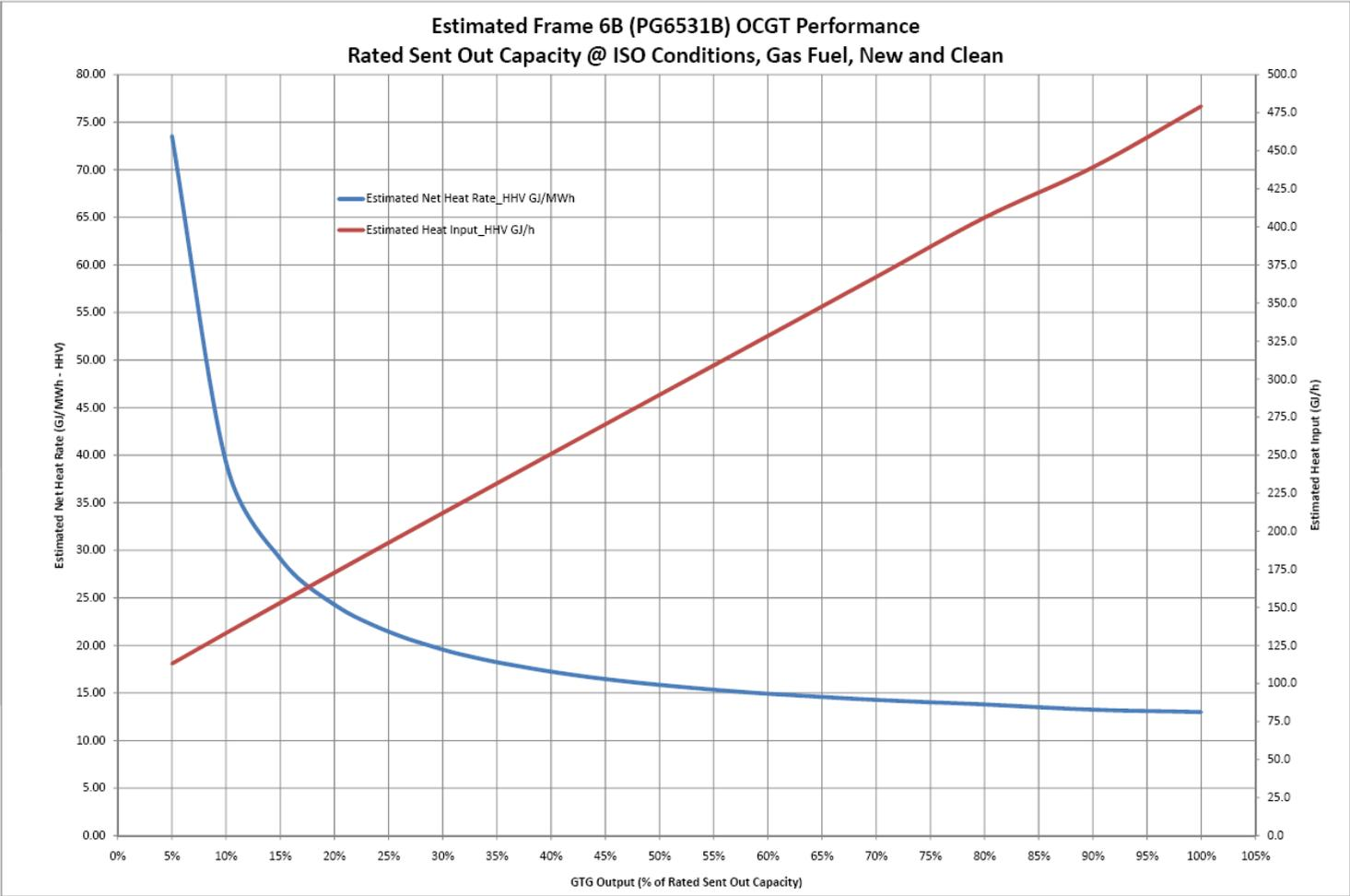
An example heat input function and resulting average heat rate curve are provided in Figure 5. The marginal heat rate at any level of output is defined as the gradient of the heat input curve. It should be noted that the marginal HHV heat rate is typically lower than the average HHV heat rate at maximum sent-out rated capacity.
