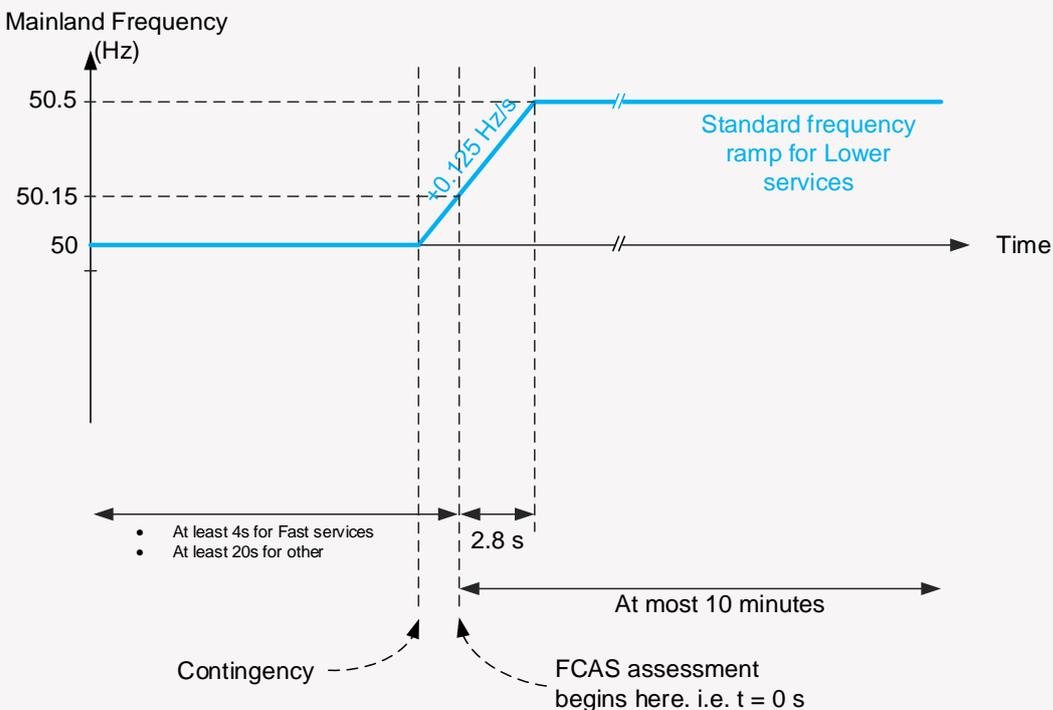
**Figure 2 Standard Frequency Ramp for Tasmania**
