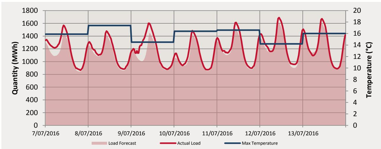
The maximum temperatures for this trading week ranged from 14.2°C to 17.4°C. The actual load peaked at 1689.983 MWh on the 12/7/2016.
