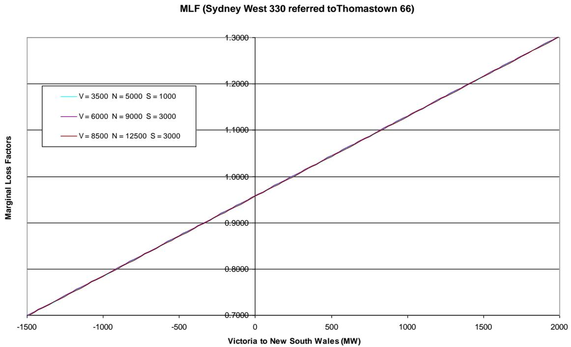
FIGURE 1: MARGINAL LOSS FACTOR VS TRANSFER FOR VIC-NSW NOTIONAL INTERCONNECTOR
