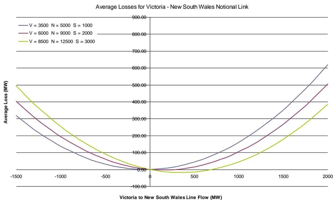
FIGURE 3: AVERAGE LOSS VS TRANSFERS FOR VIC-NSW NOTIONAL INTERCONNECTOR
