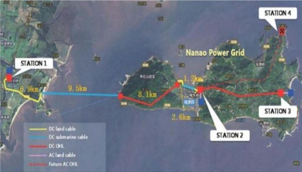
Figure 2: Nan’ao multi-terminal VSC-HVDC project (from [20]).
