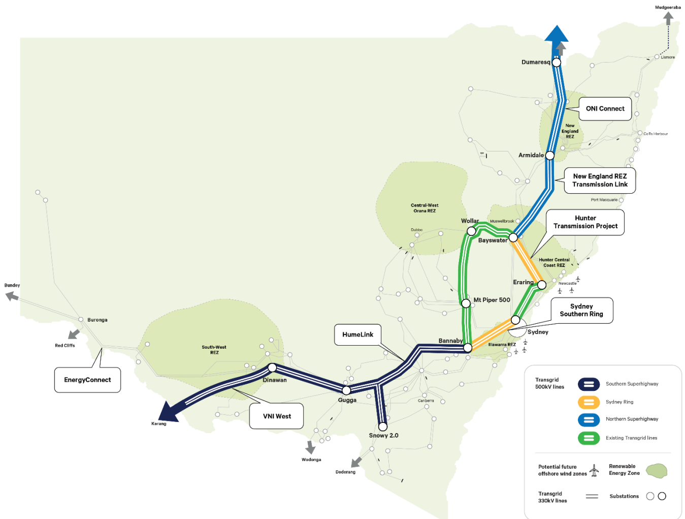
Figure 2: The NSW 500 kV Energy Superhighway
