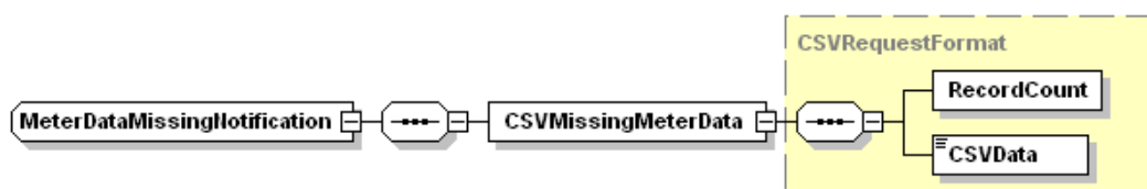
FIGURE 4-8 METERDATAMISSINGNOTIFICATION ASEXML SCHEMA
