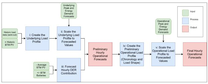
Figure 4: Overview of load forecasting process
