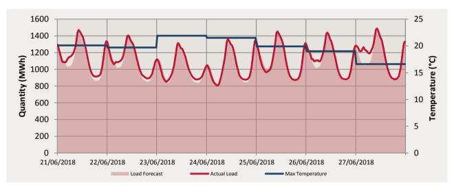
The maximum temperatures for this trading week ranged from  $16.6^{\circ}$ C to  $21.9^{\circ}$ C. The actual load peaked at 1488.18 MWh on the 27/6/2018.
