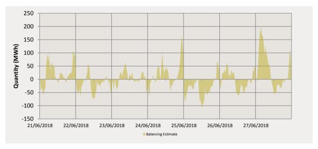
The majority of the balancing activity this week occurred within Balancing Demand. The maximum balancing demand for the week reached 199.2925 MWh on the 27/6/2018. The maximum balancing supply for the week reached -109.942 MWh on the 25/6/2012.
