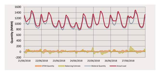
Total balancing supply equalled -5228.15 MWh whereas total balancing demand equalled 6796.541 MWh. The Total STEM Traded quantity was 13276.364 MWh, with the STEM Clearing Quantity ranging between 7.905 MWh and 87.64 MWh.
