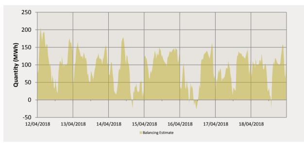
The majority of the balancing activity this week occurred within Balancing Demand. The maximum balancing demand for the week reached 206.483 MWh on the 12/4/2018. The maximum balancing supply for the week reached -26.921 MWh on the 16/4/2012.
