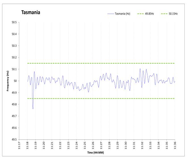
Figure 1: Low Frequency Normal Event in Tasmania refer to item 1 in Table 2 with the frequency exceeding the Tasmania Frequency Operating Standard
