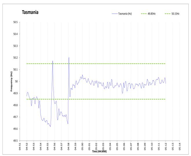
Figure 7: Low Frequency Normal Event in Tasmania refer to item 3 in Table 2 with the frequency exceeding the Tasmania Frequency Operating Standard
