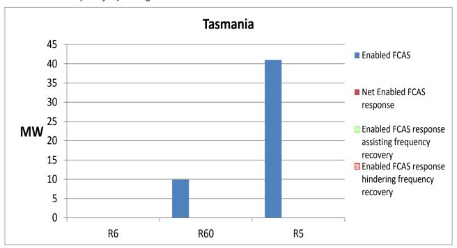
Figure 2: FCAS response to Normal (Non-Contingency) Low Frequency Event on 2<sup>nd</sup> July 2011.
