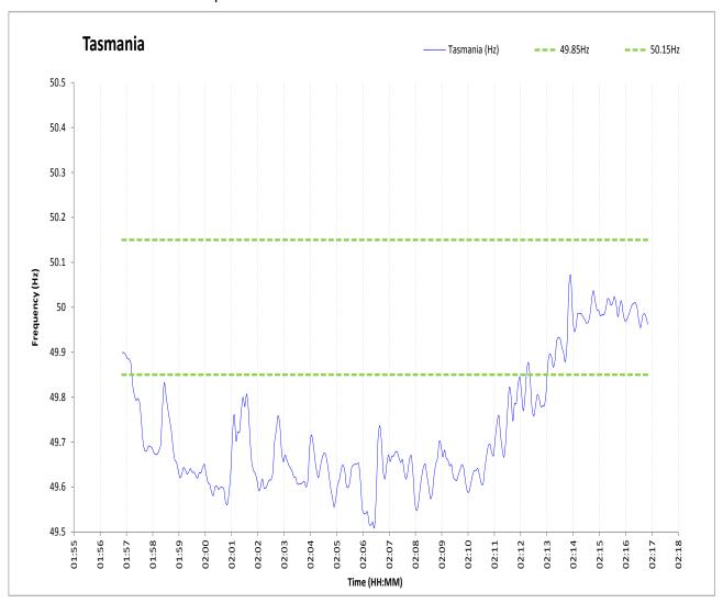
Figure 3: Low Frequency Normal Event in Tasmania refer to item 2 in Table 2 with the frequency exceeding the Tasmania Frequency Operating Standard
