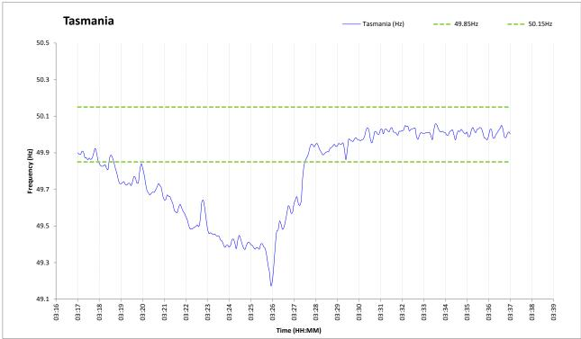
Figure 5: Low Frequency Normal Event in Tasmania refer to item 3 in Table 2 with the frequency exceeding the Tasmania Frequency Operating Standard
