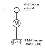
**Description of connection point:** *Small resource connection point* comprising a 4 MW exempt battery (small BDU)
