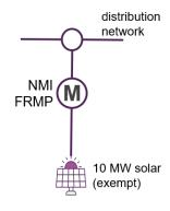
**Description of connection point:** Small resource connection point comprising a small generating unit (exempt via application to AEMO)
