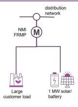
**Description of connection point:** Large customer connection point with exempt generation onsite (NOT a *small resource connection point* as there is load onsite unrelated to the small bidirectional unit/small generating unit), all net generation sold to retailer
