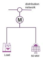
**Description of connection point:** Registered *integrated resource system* (generating unit + load) connected to a *distribution network*
