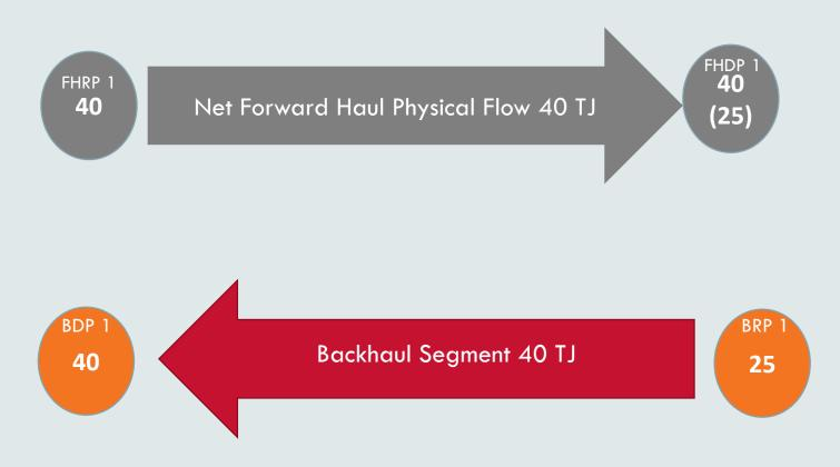
In this case where the backhaul receipt point is also a forward haul receipt point, a maximum of 25 TJ can be backhauled between BRP 1 and BDP 1 (i.e. it is constrained by the amount of spare physical capacity at BRP 1 because only 25 TJ of gas can be injected at that point)
