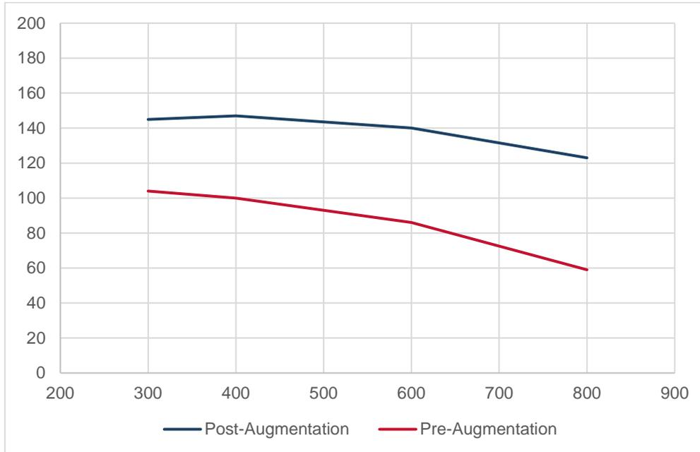
Figure 3 SWP withdrawal capacity pre- vs post-augmentation for varying system demands (2017 VGPR)
