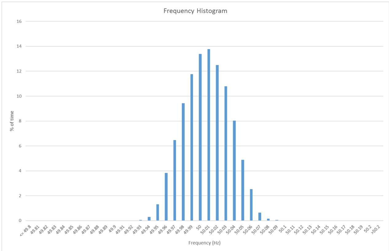
The frequency performance of the SWIS for the period under review is provided in Figure 1. The frequency remained in the normal operating band for 99.996% of the time. This meets the Frequency Operating Standards specified in the Technical Rules. This performance was a product of the combination of active frequency control via AGC of the LFAS generators and the governor responses from all online generators.
